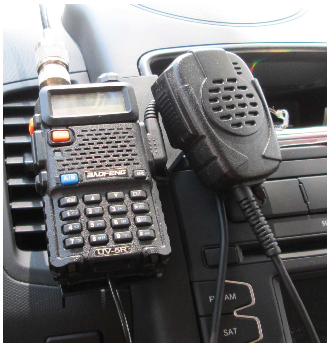
The finished instal has the UV-5R over the vent with the mic clipped to the cable.....
