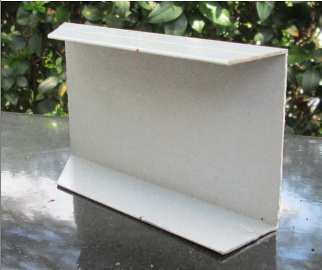
The 3" aluminum channel above was scrap from building our cabana. Sides are 1.5" ID is 3".
